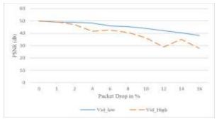
Figure 6. Packet drop Vs PSNR (low and High Motion Video)
