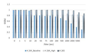
Figure 14. Effect of Jitter over video codec in terms of SSIM index
