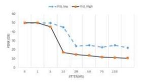
Figure 11. Effect of jitter over PSNR for low and high motion video
