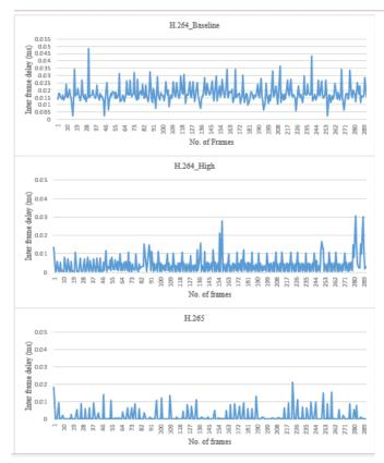
Figure 10. Comparison of Jitter performance for different video codec
