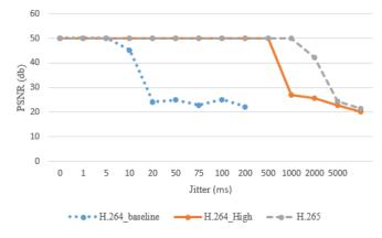
Figure 13. Effect of Jitter over video codec in terms of PSNR
