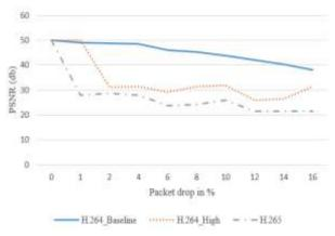
Figure 8. Packet drop Vs PSNR for different video codec
