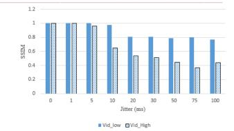
Figure 12. Effect of Jitter over SSIM index for low and high motion video
