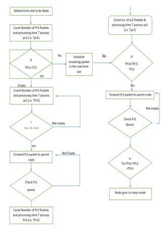
Figure 2: Power and QoS Efficient Algorithm Design
