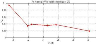
Figure-11 Simulation result for Probability of missed Detection w.r.t NFR
