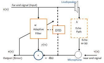
Figure-1 A Typical DTD based Acoustic Echo Canceller
