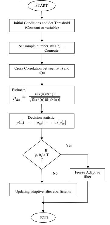
Figure-2 Flowchart for cross correlation based Double Talk Detector
