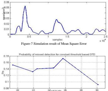
20 22 24 <sub>NFR(dB)</sub> 26 28 30 Figure-8 Simulation result for Probability of missed detection w.r.t NFR
