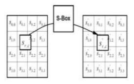
Fig 2:SubBytes( ) applies the s-box to each byte of the state.
