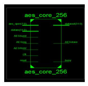
Fig 9:AES RTL Structure
