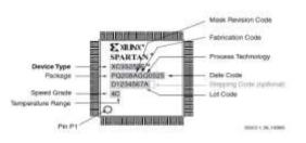
Fig. 5 Spartan 3 QFP package
