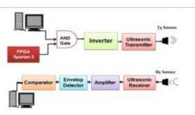
Fig.1 Block Diagram of an Underwater Acoustic Modem
