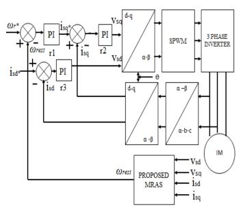
Figure 2.Sensorless indirect field oriented control with proposed speed identification block
