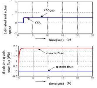
Figure6.(a)Actual speed and estimated speed[rad/s] versus time[s] (b)d-axis and q-axis rotorflux[Wb]
