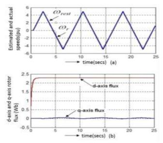
Figure5.(a) Actual speed and estimated speed [rad/s] versus time [s]. (b)d-axis and q-axis rotor flux[Wb]
