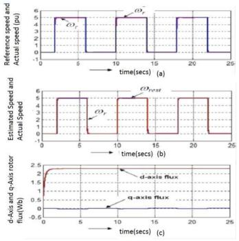
Figure 4 (a) Reference speed and actual speed [rad/s] versus time [s]. (b)Actual speed and estimated speed [rad/s] versus time[s](c) d-axis q-axis rotor flux [Wb] versus time[s].
