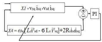
Figure 1. Model Reference Adaptive Control (MRAC) speed estimation
