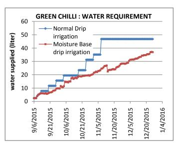
Figure 4: Water requirement of green chilly for normal and moisture based irrigation
