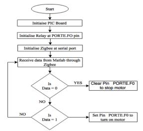
Third node consists of microcontroller PIC 16F877A along with Zigbee module, relay and AC motor. Command sent by controlling node is received by PIC microcontroller. As per command received, it will turn ON and OFF the motors in farm area.
