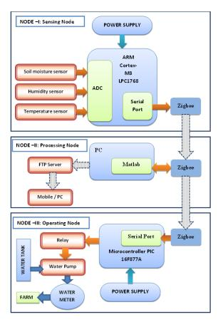
Figure 1 : Block Diagram
