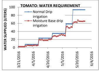
Figure 3: Water requirement of tomato for normal and moisture based irrigation
