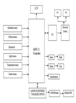
Fig 1: Block Diagram of the System
