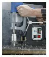
Fig 1.A magnetic core drill machine making hole.
