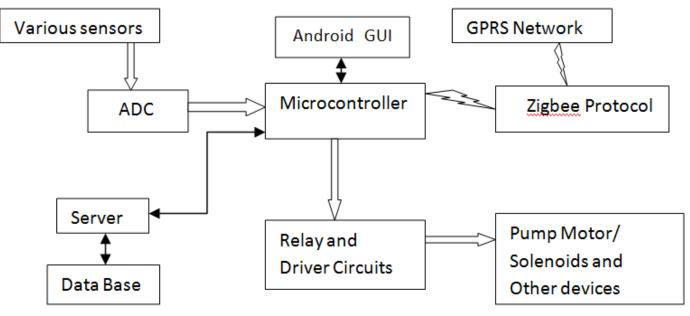
Fig 2: System Architecture for Automated Irrigation System
