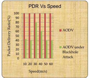
Figure 15:PDR Vs Speed of Nodes
