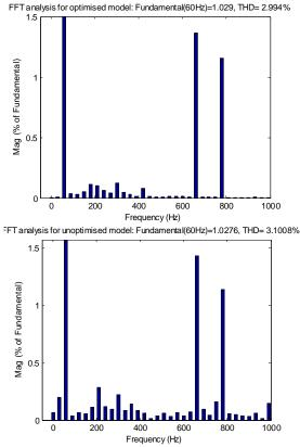
Figure 5: (a) optimised harmonics (b) un-optimised harmonics
