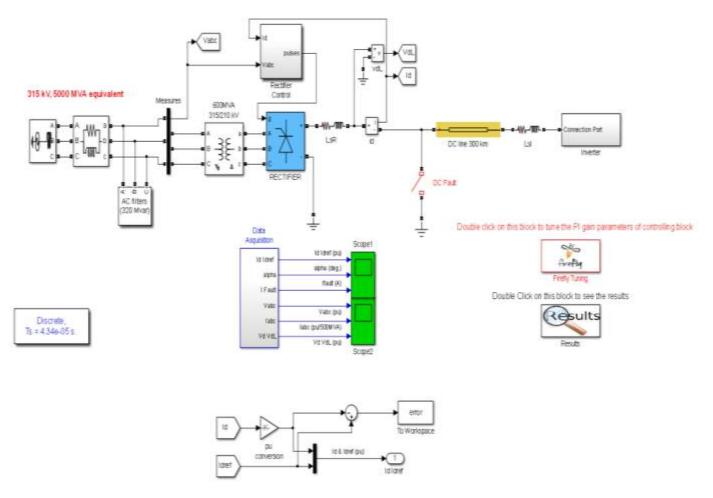
Figure 3: HVDC simulink model with its controller
