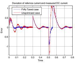
Figure 6: deviation of observed DC current to reference in optimised and un-optimised case
