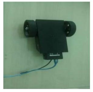
Figure 3. Wheelchair prototype for SSVEP based BCI control
