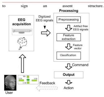
Figure 1. Conceptual block diagram of the proposed SSVEP based wheelchair control system.
