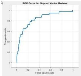
Fig 4.6: ROC Curve of the SVM Classifier after training, Showing more than 90% of area under the curve (AUC)
