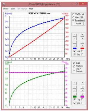
Figure-20: The graph of Impedance v/s Frequency
