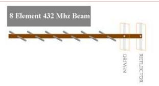
Figure-2: 8 element Quagi antenna
