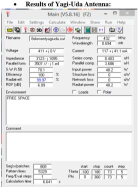
Figure-3: Input power, SWR and radiating efficiency of Yagi-Uda antenna
