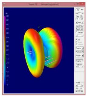
Figure-8: The multi-colour 3D radiation pattern
