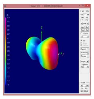
Figure-17: The multi-colour 3D radiation pattern
