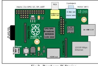
Fig 2. Raspberry Pi Device
