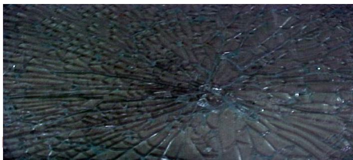
Glass broken into finer particles during quenching
