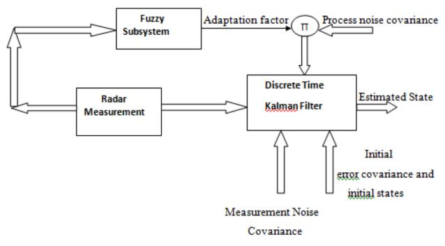
Figure 2 block diagram of fuzzy kalman filter
