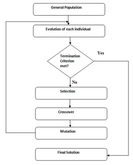
Figure 1 Flow Chart Of Genetic Algorithm
