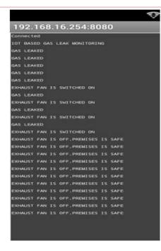
Fig-4 Notifications on User's Mobile via TCP/IP Client
