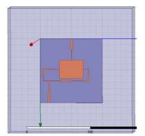
Figure 1.Patch antenna with power divider
