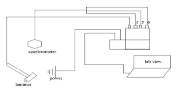
Fig1: Experimental setup line diagram
