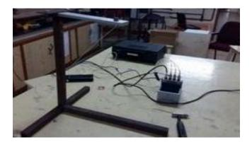
Fig3: Experimental setup for cantilever beam
