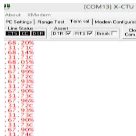
Figure 9 Reading of Remote Sensor in XCTU received by Zigbee Receiver
