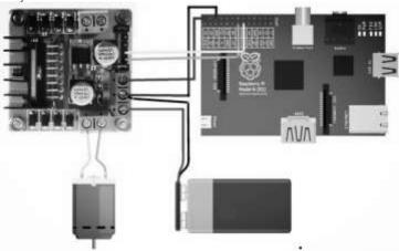
Figure 3 Connection of Raspberry Pi with L298N motor driver[9]
