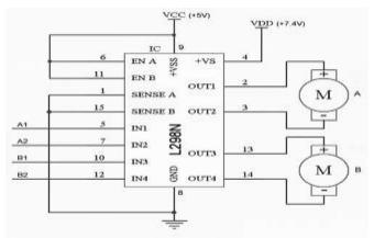
Figure 4 Circuit Diagram of Connection of motor driver with motors[10]
