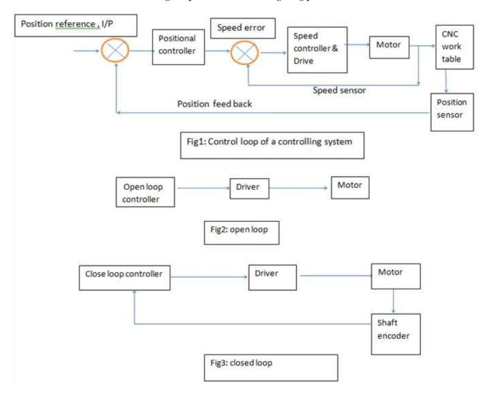
Servo motor, Motor Drive, Gear Box, Actuator, Feedback Encoder, Motor control, Control of turning software and Drive communication software.
