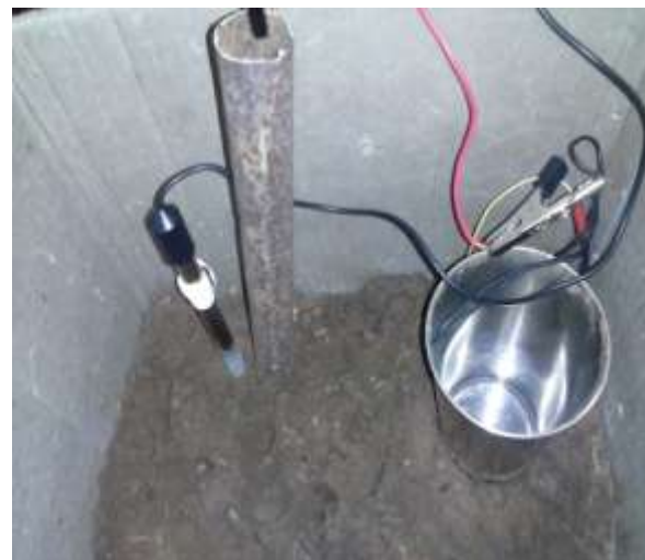
Figure9. Corroded steel as working electrode
