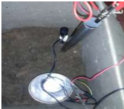
Figure6. Three electrode cell using non-corroded steel
