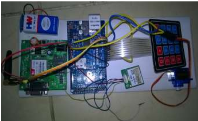
Fig.5 Arduino interfaced with GPS,GSM, keypad, servo
