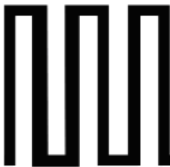
Fig.1 Meander Line Structure
