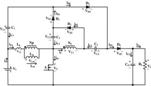
Fig 2Circuit configuration of the high-step-up converter
