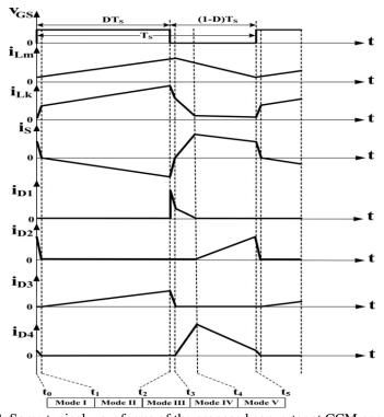
Fig. 3: Some typical waveforms of the proposed converter at CCM operation
