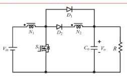
Fig.1 Conventional high step up dc-dc converter
