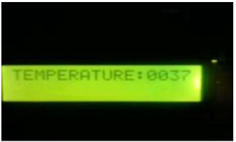
Figure 8. Temperature Sensor at 37° c
