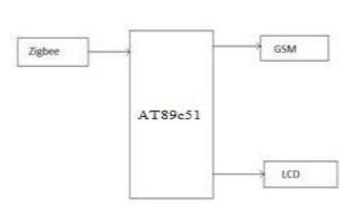
Figure 2.Receiver Section.
