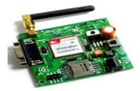
Fig.5: GSM SIM900A Modem
