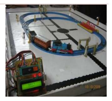
train passes Sensor2 positioned prior to gate, a signal is sent to the controller indicating the approaching train. The controller then sends a signal to the gates assembly, causing the gate arms on either side of the road to close. When the train finally has passed Sensor3, which is positioned just beyond the gate crossing section, a corresponding signal is sent to the controller, which in turn triggers both the gate arms to open simultaneously.
