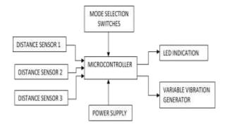
Fig.3.1 Block Diagram of System
