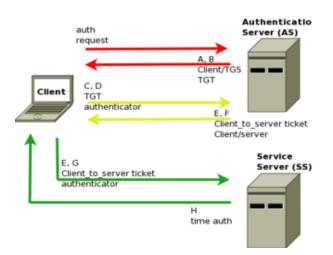
Figure 2. Kerberos authentication process
