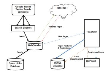
Fig.3. System Architecture
