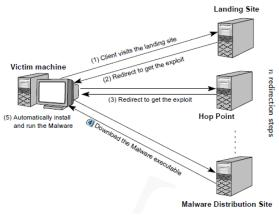
Fig. 2.1: A typical Interaction with of drive-by download victim with a landing URL.
