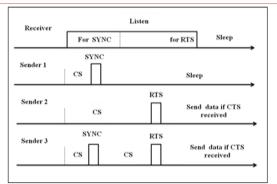
Fig-2: Timing Relationship between a Receiver and Different Senders
