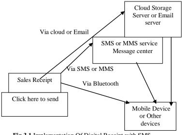
Fig 3.1 Implementation Of Digital Receipt with SMS, Bluetooth, Cloud And Email
