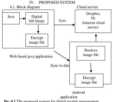
fig: 4.1 The proposed system for digital receipt management system
