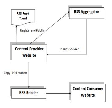
Figure 2. RSS Producer-Consumer architecture
