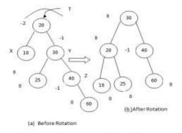
Fig.4 :AVL property is destroyed by insertion of 60. AVL property is fixed by left rotation
