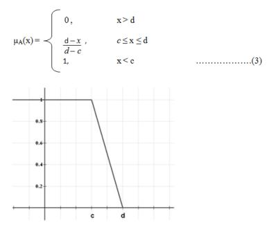
Figure 1.4: Linear representation down membership function
