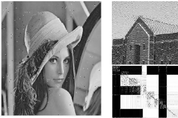
Figure 7. Average Filtering attack (5X5) a) Attacked Host Image b) Extracted Primary Watermark1 c) Extracted Secondary Watermark2
