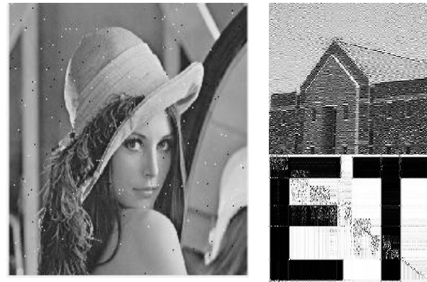
Figure 6. Salt & Pepper noise a) Attacked Host Image b) Extracted Primary Watermark1 c) Extracted Secondary Watermark2
