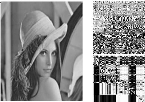
Figure 8. Median Filtering attack a) Attacked Host Image b) Extracted Primary Watermark1 c) Extracted Secondary Watermark2
