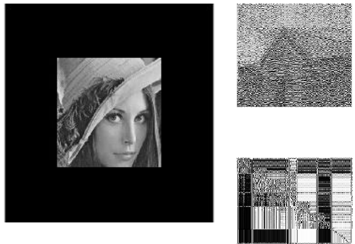
Figure 11. Cropping attack (50% area remaining) a) Attacked Host Image b) Extracted Primary Watermark1 c) Extracted Secondary Watermark2
