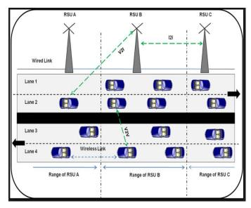
Figure1 Vehicular Ad hoc Networks configuration
