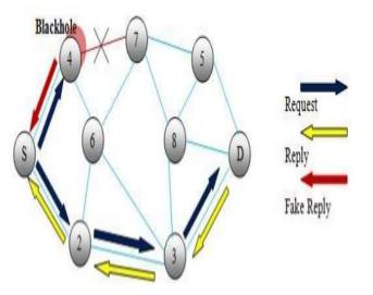
Figure3 Black hole attack diagram
