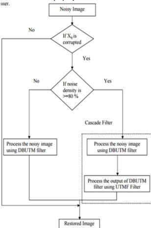
Figure 4 Flow chart of the proposed noise removal scheme
