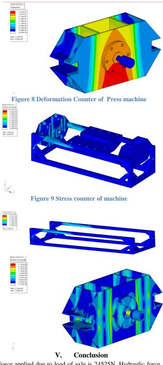
Force applied due to load of axle is 24525N. Hydraulic force acting on piston and cylinder is 490500N. To check the effects of maximum forces on the designed structure a Linear static Analysis is carried out by using Finite Element Analysis Technique.
