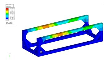
**Figure 7 Deformation Counter of Frame**
