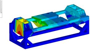
Figure 6 Deformation Counter of Machine
