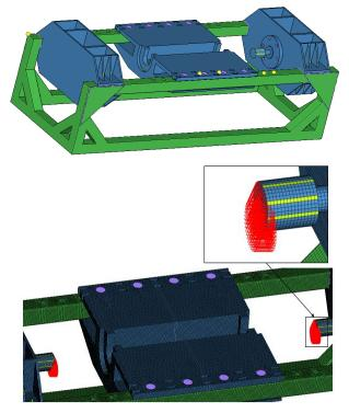
Figure 4 Loading Condition on Press Machine
