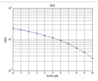
Figure 5. Plot of bit error rate versus  $E_b/N_0$  for  $E_b/N_0$  from 0 to 10 dB using binary phase shift keying.
