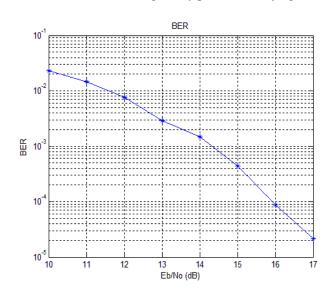
Figure 6. Plot of bit error rate versus  $E_b/N_0$  for  $E_b/N_0$  from 10 to 20 dB using binary phase shift keying.
