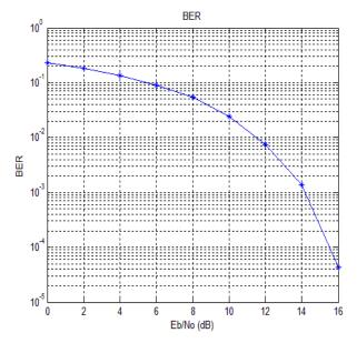
Figure 4. Plot of bit error rate versus  $E_b/N_0$  for  $E_b/N_0$  from 0 to 20 dB using binary phase shift keying.
