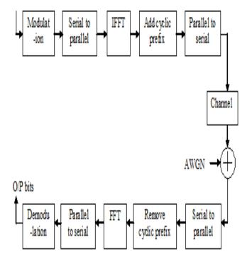
Figure 2. Block diagram of orthogonal frequency division multiplexing transmitter and receiver.
