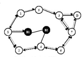
Fig.2. Network flooding by RREQ messages
