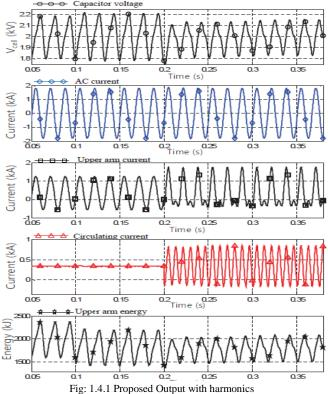
Figure 1.4.2 illustrate the outcome of different component in circuit the top most waveform illustrate capacitor voltage where as respectively from top second is AC current waveform in kA ,upper arm current, circulating current , and upper arm energy.
