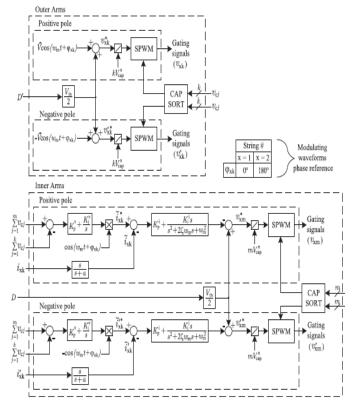
Figure: 1.3.4 Proposed control loop each string is compensated by SVPWM.
