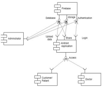
2. Component level diagram for proposed system
