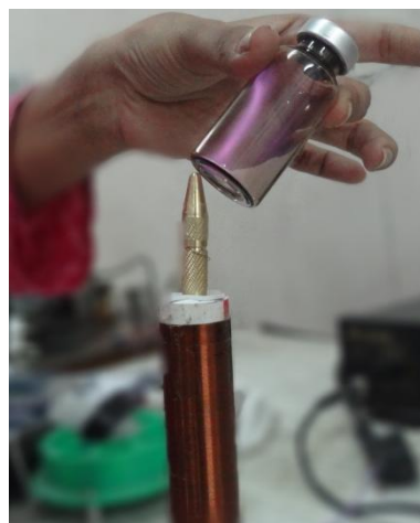
Fig 6 : Using Hand as GND Electrode
