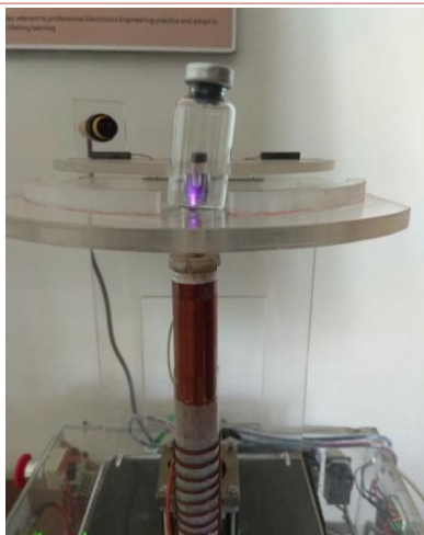
Fig 8 : Plasma in Sealed Vial
