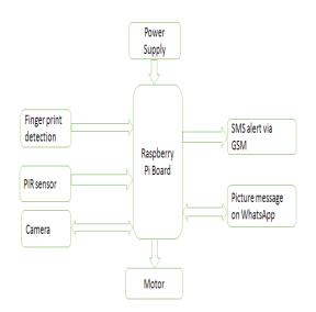
Fig.1 Block diagram of Whatsapp/Telegram Controlled Advanced Security System
