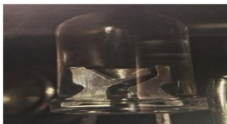
Figure 8: A 4x zoom photo of an ultra-violet LED has been shown in picture
